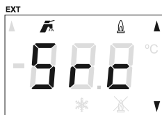
Fig. Service required display
