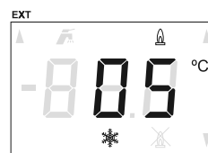
Fig. Frost protection is activated
